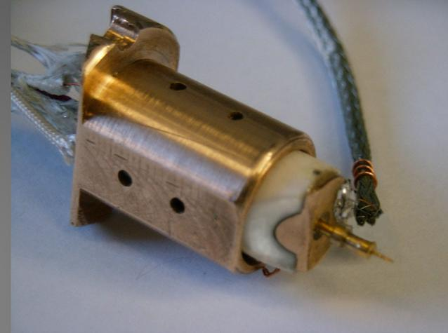
Piezo scanner with probe
