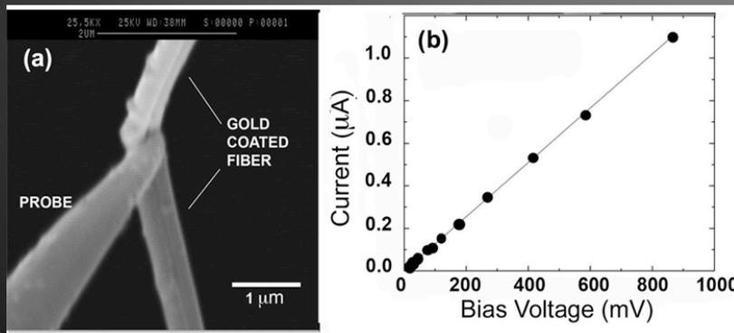
**Fiber based gold nanowires probed by an STM tip**
