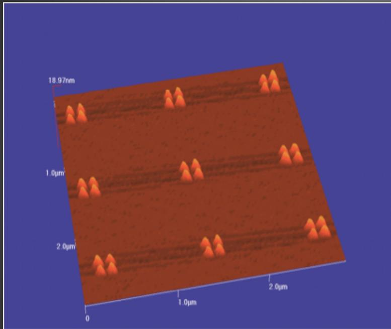
**AFM topographic image of 30 nm wide 115 nm spaced gold nanopads**
