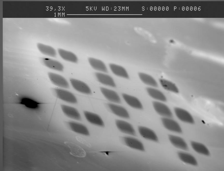
Micropositioning of shadow mask yields Pt thin film patterns. Layer thickness approx 5-10 nm
