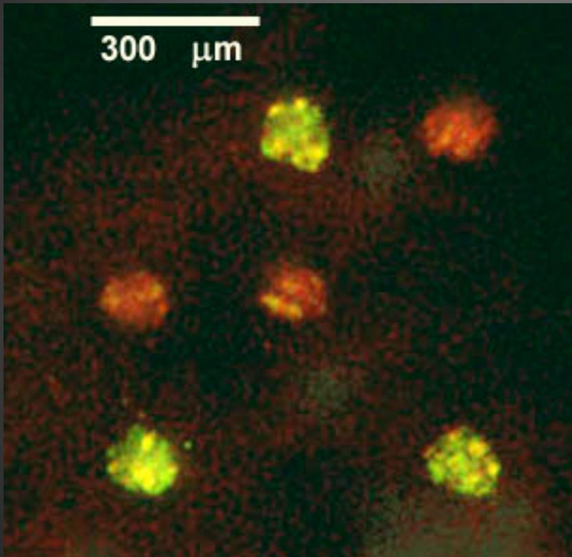
Two different antigens have been deposited in monolayers on six arbitrary locations of a 3x3 array. The remaining three locations have been coated by platinum layers for control. The device is incubated for 20 min. in a solution containing the antibodies specific for the two deposited antigens. The antibodies are tagged with fluorescent molecules of different colours, which make the antigens visible when they bind their antibodies
